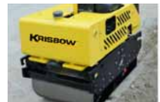
Side and curb clearance allow for the closest approach to curbs walls and other obstacles
